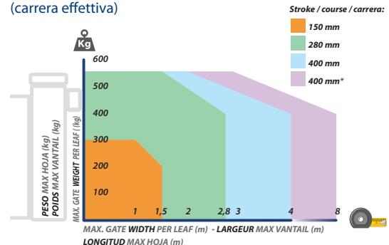
The gate structure, design (solid, in-filled), height and strong wind pressure may affect and decrease the indicated values. Make always sure the gate structure is adequate to automation.
