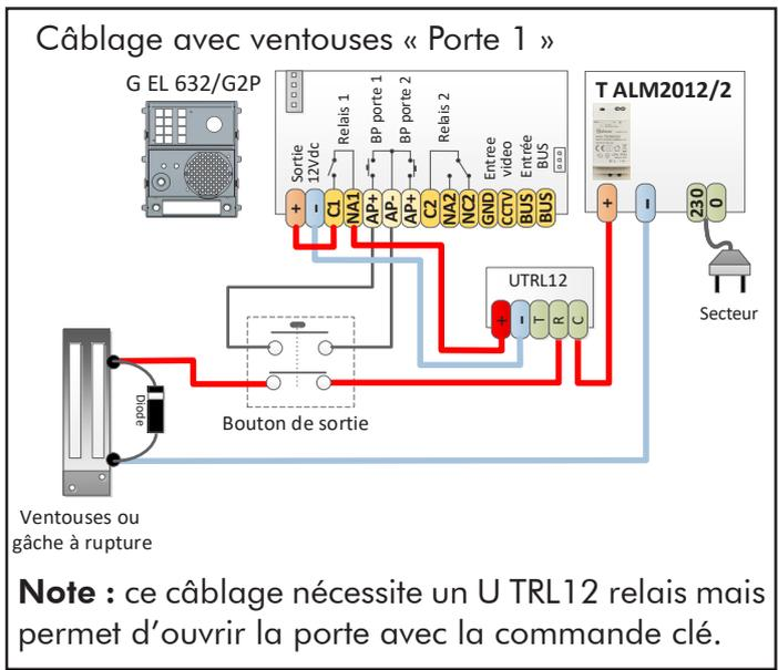
SCHEMA RACCORDEMENT PLATINE NEXA
